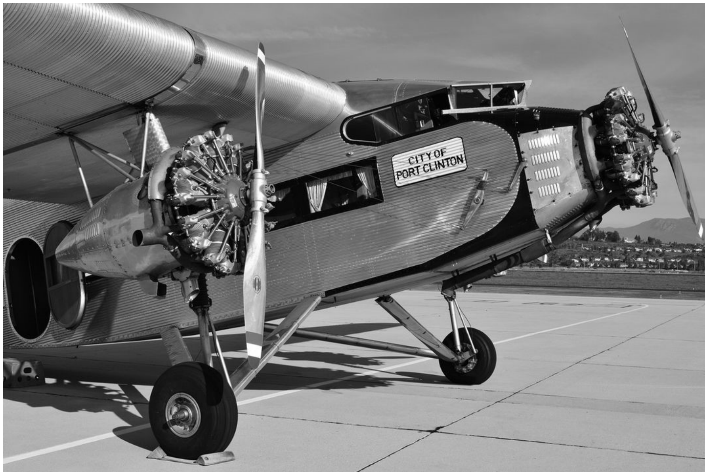
The Ford Trimotor was the first popular civil design to use then-new radial engines.
